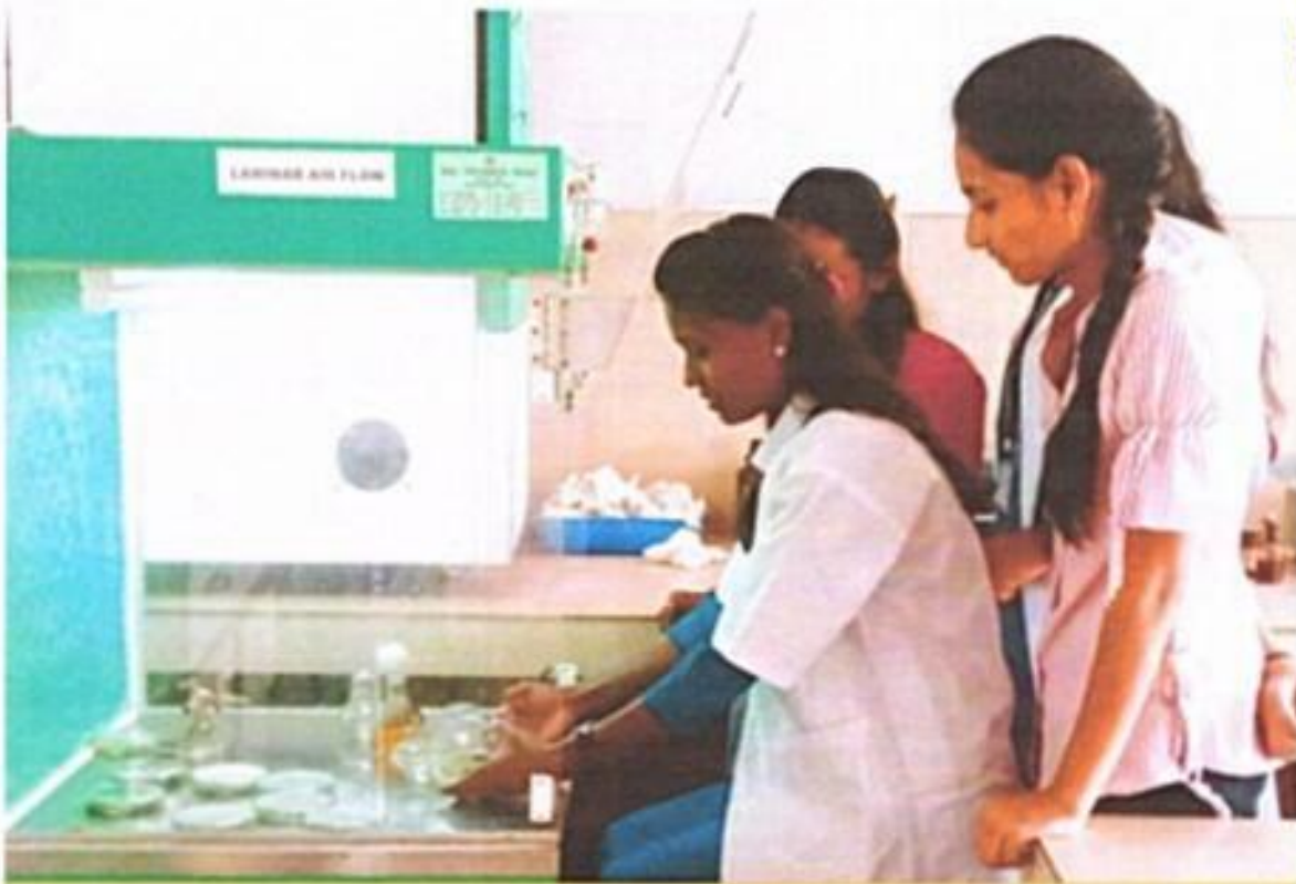
Laminar Air Flow Cabinet
